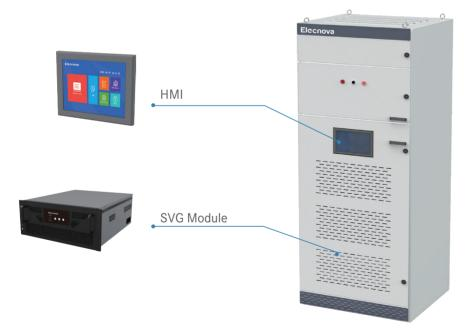
SFR-SVG is a new-generation product of Static Var Generator(SVG), it used the latest technology application for the reactive power compensation. When the SFR-SVG parallel in the grid, it equalized as a dynamic reactive current source. The reactive current of the SVG could be flexibly controlled and compensate the reactive power automatically.
