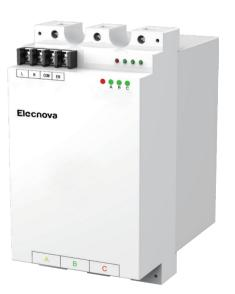
LBT series dynamic switching unit refers to a kind of contactless rapid switch with high reliability, and it is used in dynamic power factor compensation equipment. Particularly apply to switching occasions requiring rapid and no-wearswitching. It is usually applied into occasions where reactive change is frequent, such as lifting equipment, elevator and electric welding machine.
